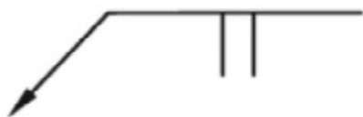
Figure-1: Square Groove Welding Symbol
