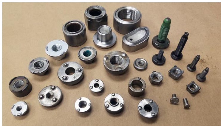
Figure-1 – Projection weld nuts - Examples
