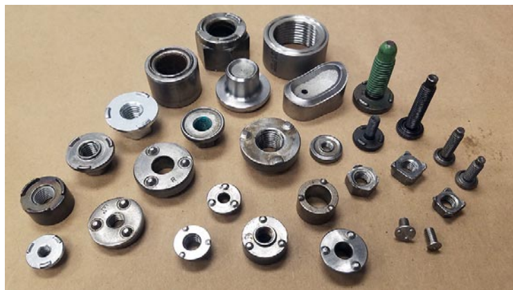
Figure-1 – Projection weld nuts - Examples
